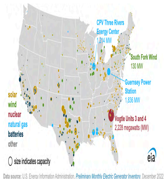
Figure 42. Planned 2023 U.S utility-scale electric generator additions.
