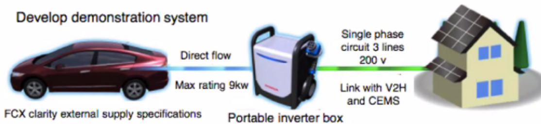
Figure 18. Powering a house with an FCEV in case of a shut-down. Source: Jammes.L. 2021.
